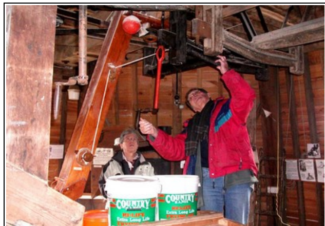
Setting the gap between the stones
